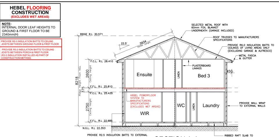
PROVIDE R2.5 INSULATION BATTS TO EXTERNAL WALLS OF LIVING AREAS ONLY (INCLUDING WALLS BETWEEN GARAGE & LIVING)
